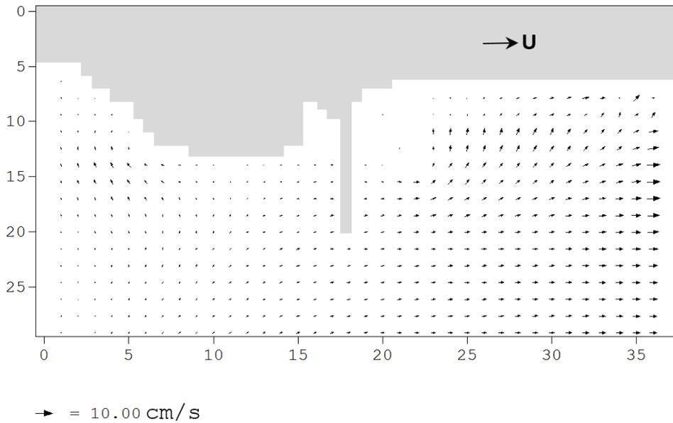
Figure 3. Current profile at the port area during the spring tide
